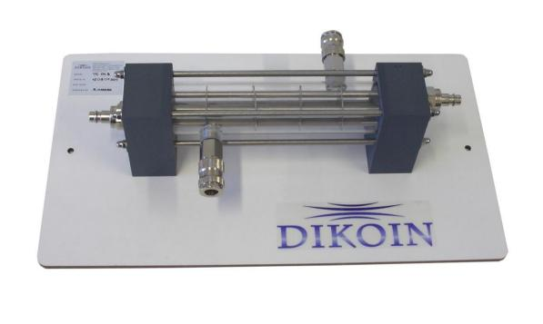
Optional Accessory: TC 01.3 - SHELL TUBE HEAT EXCHANGER The shell tube heat exchanger is one of the most widely used in the industrial sector.
