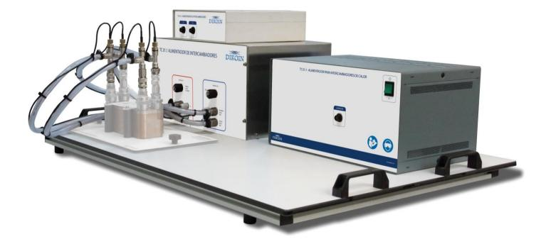
The TC 01.1 equipment is the core of the whole heat exchanger. TC 01.1 is the module that provides hot and cold water to the heat exchangers, in addition to measuring the temperatures and flow rates for each device.
