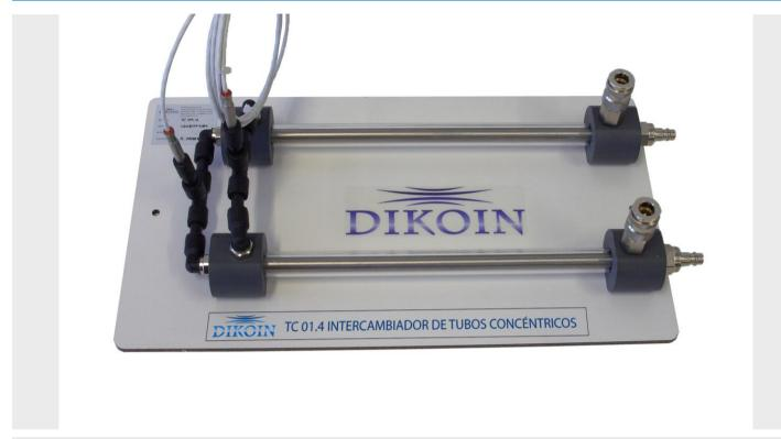
Optional Accessory: TC 01.4 - TUBULAR HEAT EXCHANGER The concentric tube heat exchanger is the simplest in design among all the heat exchangers.
